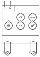
Position the device in the wall's mounting box and check cables are not interfering with the device case. Using the appropriate screw set that matches the wall box, fix the device in place without applying unnecessary torque to fixing screws.
